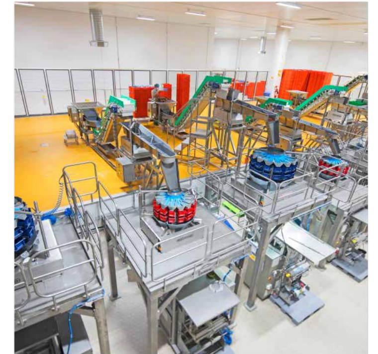
Pattyn Packaging Automation & Palletizing Robots. 6 vertical retail packaging lines, pillow pack, quattro seal, block bottom, ro-pack and Doypack
